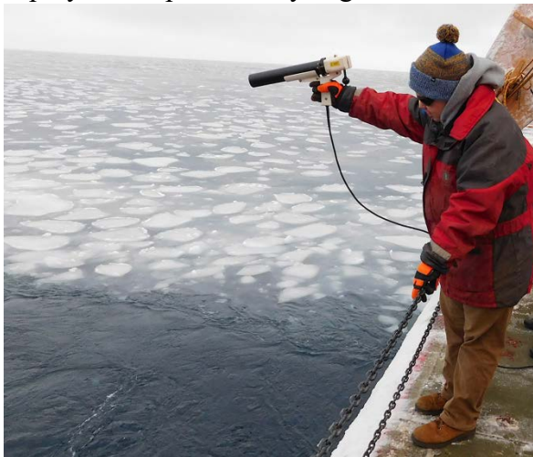
Figure 8. Deployment of an XBT to collect water column temperature data.
