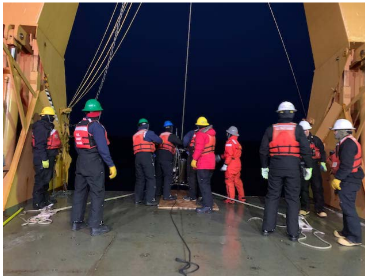
(right) Securing bottom clamp to the wire (above) Recovering the pump with tag lines used to keep the wire close to the edge of the fantail
